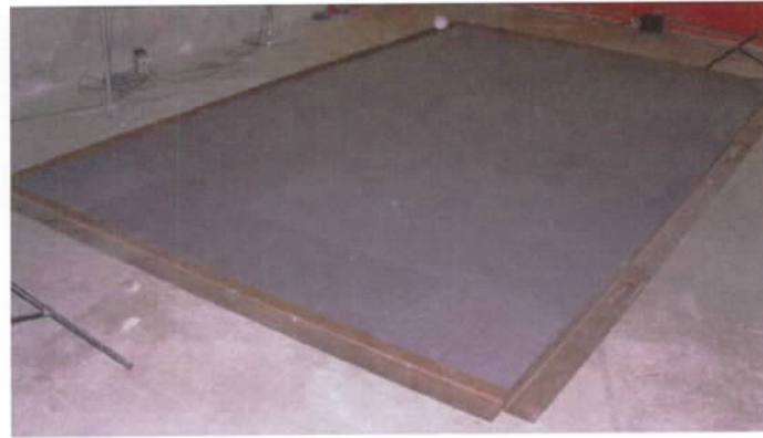
Figure 2: InterfaceFLOR Cushion Bac 746g/m 2 Carpet Tile Sample Installed in Chamber –.
